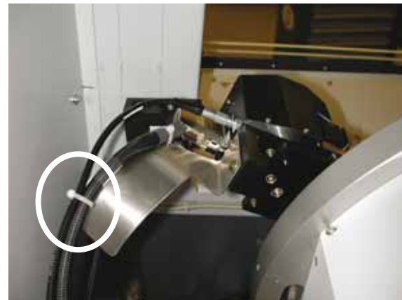
Figure 5.13 Fix power cable
