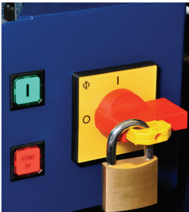
Fig. 14: System can be secured against unauthorized use by safety lock. Switch On of system is impossible when locked. All internal lines besides those marked by orange isolation are cut from electrical power supply. Generation of X-rays is impossible when system is locked.
